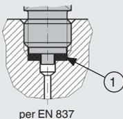
For sealing the process connections with parallel threads, flat gaskets, lens-type sealing rings or WIKA profile sealings must be used at the sealing face ①.
