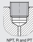
For sealing process connections with tapered threads, the sealing is made in the threads using additional sealing material, e.g. PTFE tape (EN 837-2).
