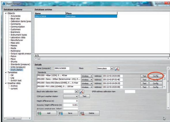
1. In the WIKA-Cal, define CPG1200 as standard in “Object manager” / “Standards (pressure)” and assign it to the workplace.
